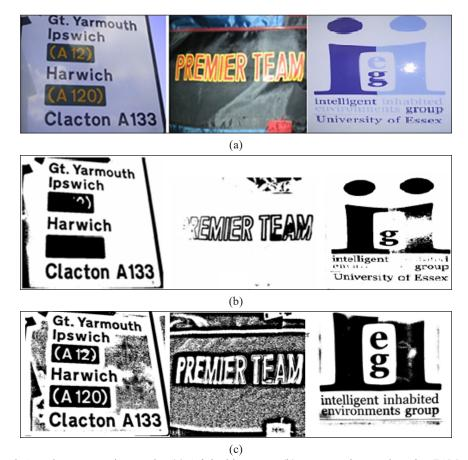
*Figure 3.* Sample segmentation results. (a) Original image set (b) segmentation results using FCM clustering and (c) segmentation results using adaptive compound binarization.
