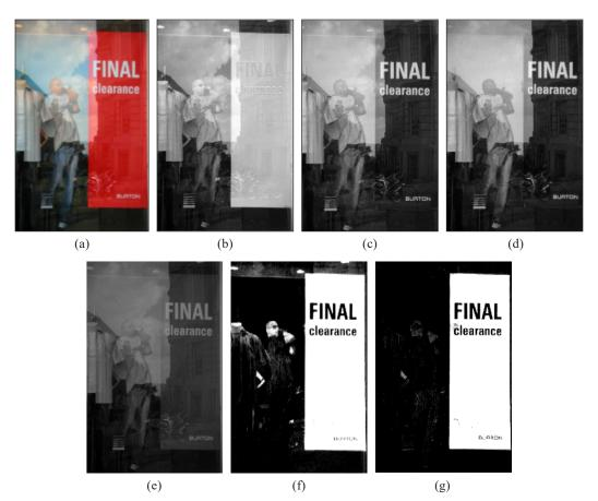
*Figure 2*. An example showing the effectiveness of the proposed image enhancement. method: (a) original image (b-d) before and (e-g) after introduction of the proposed exploited NTSC for image enhancement method according to RGB channels (red, green, blue, respectively).
